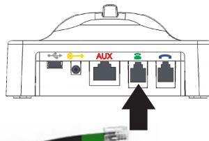
Plug one end of the telephone connector cord (green cord) into the Handset Jack of your phone. Plug the other end into the Telephone Connector Port (TEL Port) on the LH280 base
