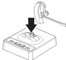
Plug in the base with the included AC adaptor. Install the battery into the headset and place in the base. Let it charge for 4 hours
