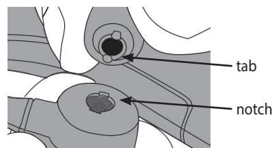
To install the new eartip, insert it into the opening in the headset, being sure to align the tabs on the eartip with the notches in the opening. Rotate clockwise to tighten
