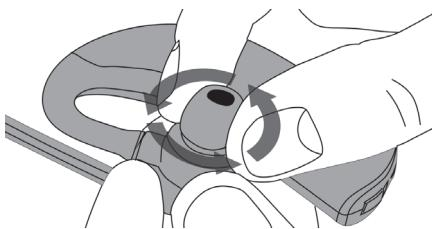
To replace the eartip, first grasp the existing eartip firmly and rotate counterclockwise to remove
