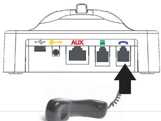
Unplug the telephone handset's curly cord from the phone base and plug into the Handset Port on the LH280
