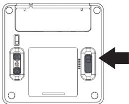
Make sure the Compatibility Switch is set correctly (most phones use setting 1). You can always call us to get the correct setting for your phone model
