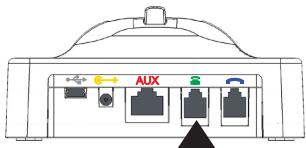
Plug one end of the telephone connector cord (green cord) into the Handset Jack of your phone. Plug the other end into the Telephone Connector Port (TEL Port) on the LH280 base
